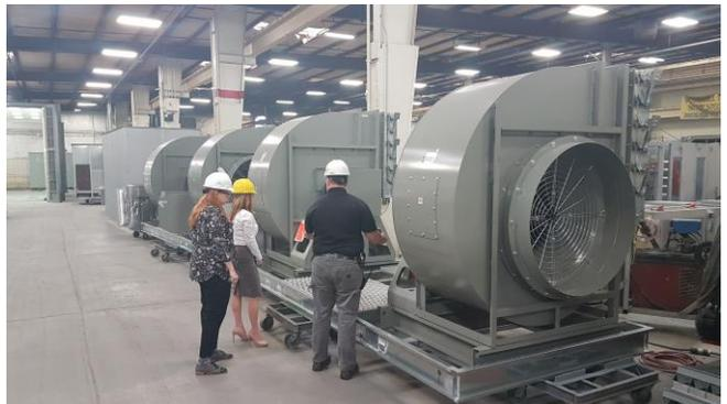
Fig 1: Tellus' air handling unit pre-assembly
