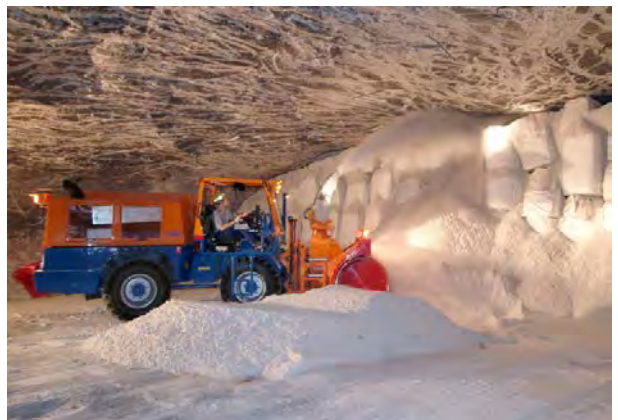
Blowing fine salt around waste packages
